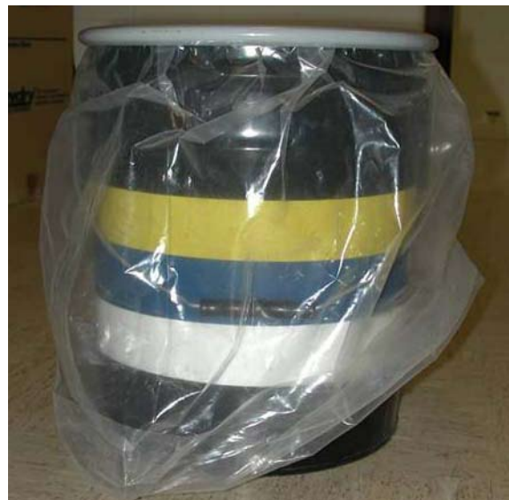
DON'T: Example of improperly stored liner
