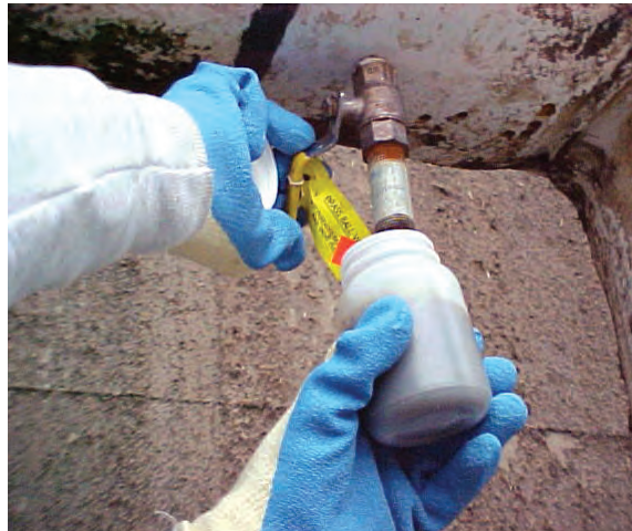
Obtaining a representative sample of liquid manure or slurry can be challenging. Most labs prefer that liquid samples fill the bottle to within an inch of the top. Installation of sampling ports with an attached hose can make sampling events much more pleasant.
